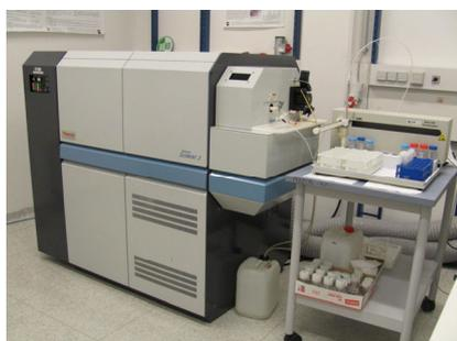
Figure 2. HR-ICP-MS instrument (Thermo Finnigan Element 2)
