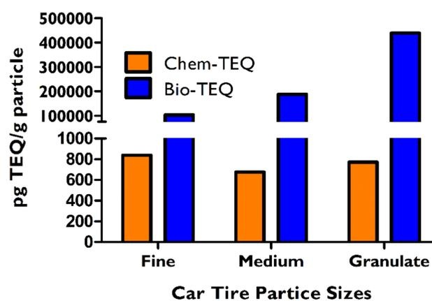
Figure 3. Comparison of Chem- and Bio-TEQ of the extracts of car tire particles. Note the difference in y-axis before and after the break.
